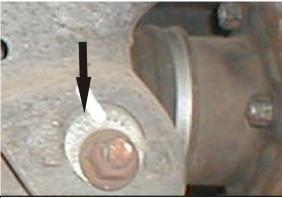
Remove the stock bushings from both control arms using heat rather than a hydraulic press to avoid accidentally bending the control arms.
