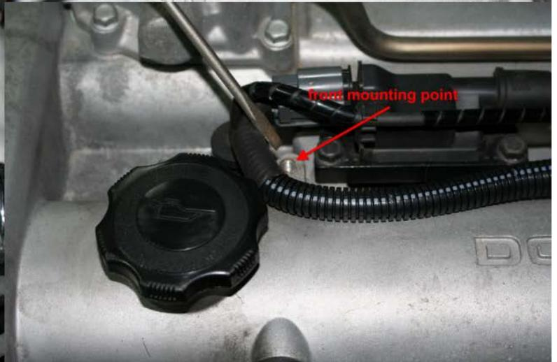
2. Place the aluminum spacers on the mounting points and line them up with the bolt holes underneath
