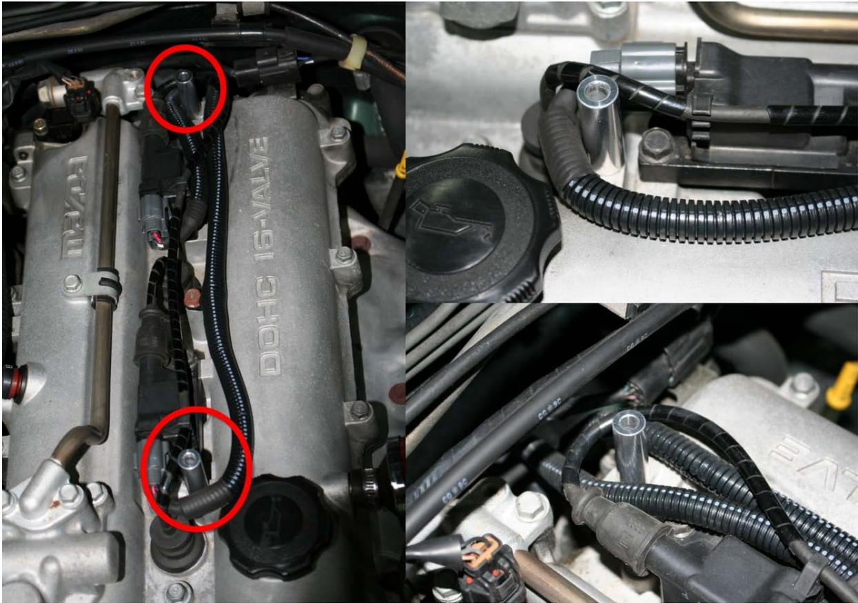
3. Fit the coil cover (notched side forward) on top of the spacers taking care to line up the bolt holes. The coil cover holes, spacer holes, and threaded mounting holes in the valve cover should be in-line
