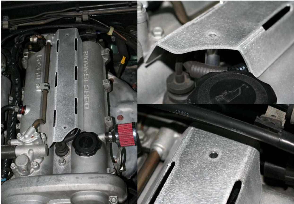
4. Find the allen bolts and install the lock washer first, then the flat washer, and slide the assembly through the cover and spacer on both the front and back mounting holes. Hand-tighten the bolts to ensure they're threaded, then use the T5 Allen head driver and tighten until the lock washer compresses. Do not overtighten as the aluminum in the valve cover might strip
