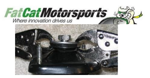
Without an impact wrench, there will be more resistance as the nut turns so you will have to use stronger means to keep the shaft from spinning. A strap wrench works well, as does a mouse pad or other thick, high-friction material held inside pliers, etc. Whatever your approach, be sure the shaft does not spin as this may damage internal seals.
