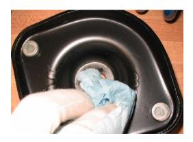
6. Support the inverted shock mount with the spring perch from your coilover sleeve. The mount should be stable. Apply the adhesive in a ring around the isolator then press it into place on the shock mount. Rotate the isolator one revolution to distribute the adhesive.
