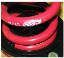
Leave spring on isolator for about an hour until glue cures
