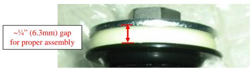
12. Ensure the gap is about 1/4" and the bushings are still centered in the shock mount.
