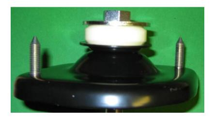
**NOTE8:** The MCU bushings need to be guided into place during tightening. The lower bushing is aided via the lower isolator and red flat washer but the upper bushing may need to be reset by hand during final tightening.
