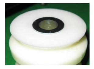
2. Place bump stop on shaft (36mm shown) followed by the round M10 Bilstein spacer (item 9). Only use one spacer per shock!
