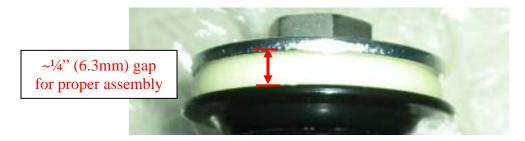
8. Ensure the gap is about 1/4" and the bushings are still centered in the shock mount. This verifies the bushings have been properly compressed.
