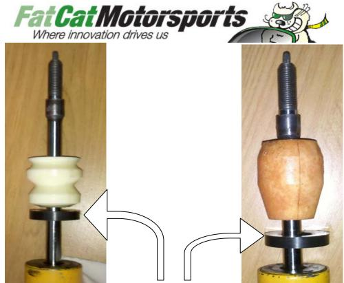
36mm stop with **bump stop spacer / packer** (arrow) 46mm stop with **bump stop spacer / packer** (arrow)
