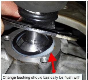
Change bushing should basically be flush with the top of the turret when the assembly is correctly installed. The wave washer will protrude, but is supposed to as it acts as a spring between the change bushing and lower shift boot
