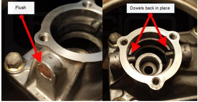
9. Now that the turret is restored to its original configuration, we will take our completed shifter assembly and reinstall it back into the turret:
