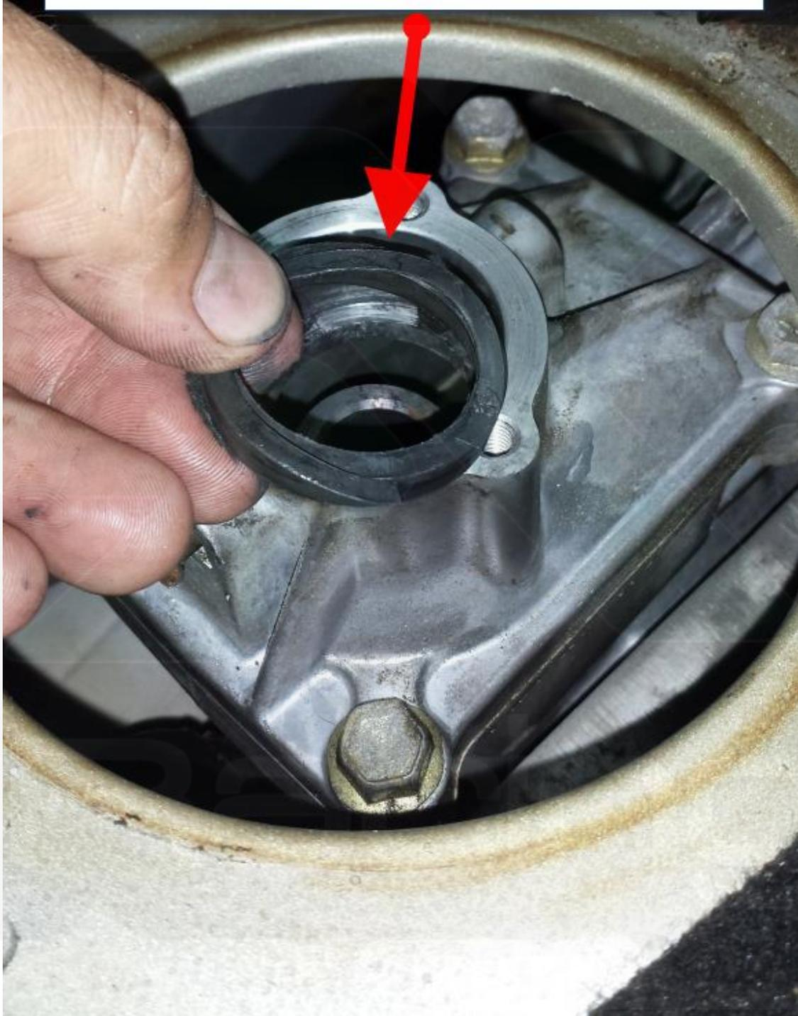
A comparison of our old change bushing and wave washer to the new ones. The wave washer was obviously broken, but the change bushing wasn't too bad. Being plastic, it should rarely fail – however - if you're replacing anything within the shifter assembly, you might as well replace everything while you're at it to fully restore the feel of the shifter!
