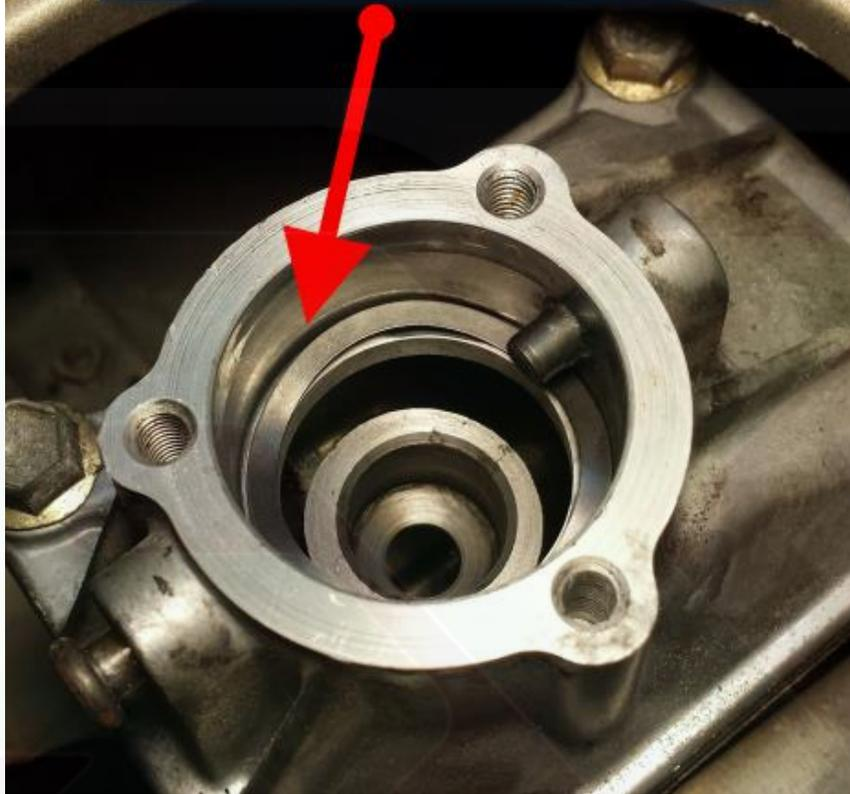
Install lower (black) change bushing on top of wave washer observing the two divot spots for the dowels
