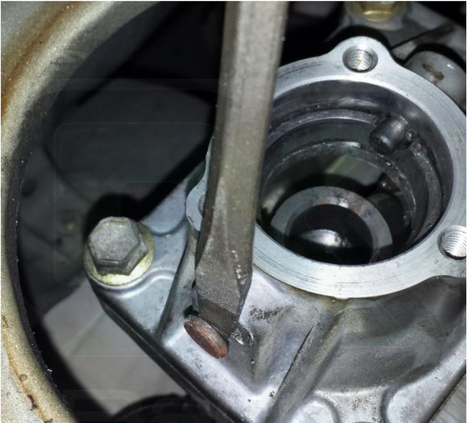
Using a flat tipped screwdriver, pry the dowel out further until it's flush on the inside of the turret wall
