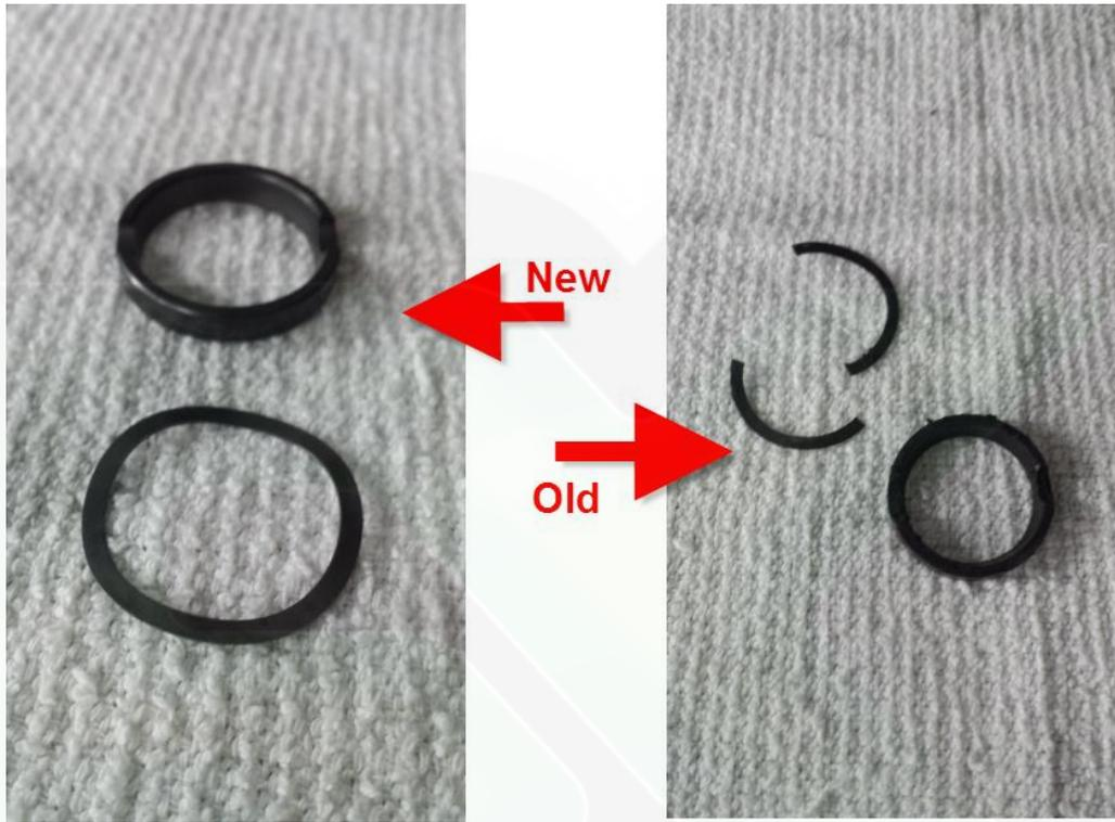
6. The next step once the lower wave washer and change bushing are removed is to go back to the shifter assembly and remove the old upper wave washer and white change bushing from the shifter. Simply remove them by sliding them upwards over the shifter shaft
