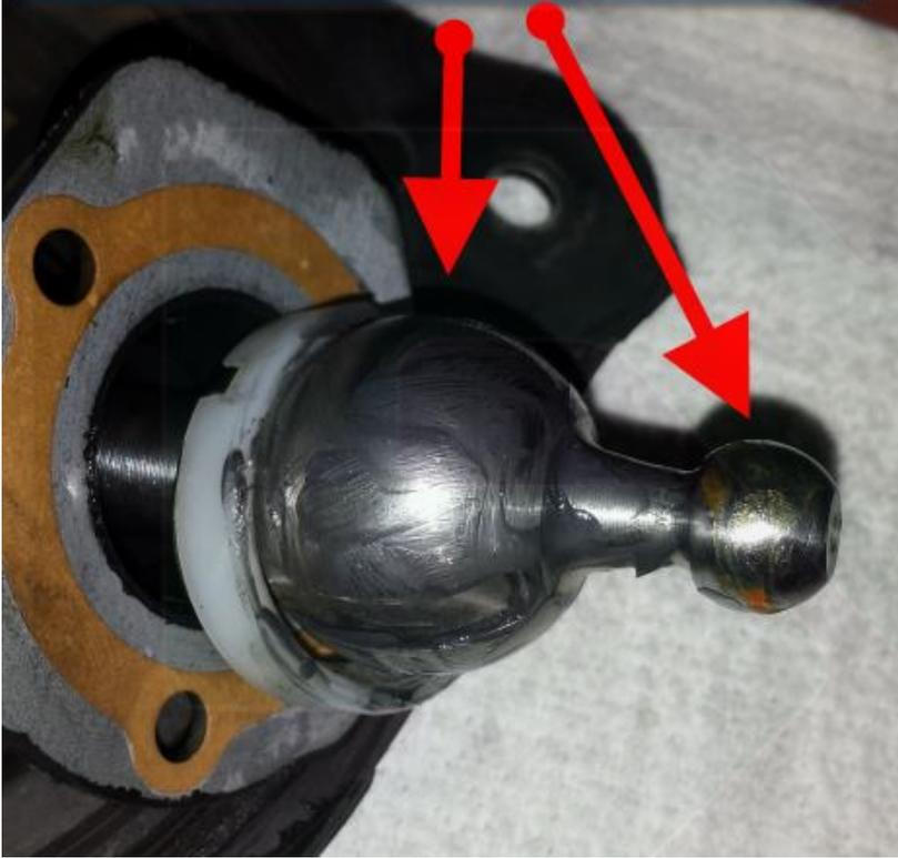
Clean the inside of the shifter turret as best you can before installing the shifter assembly!
