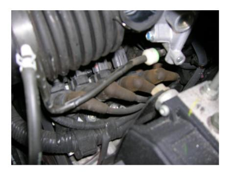
The wires are in a tight spot and are a bit of a pain to route as you change them. There is a wire loom about half way down the wires that holds all four leads, the rightmost two wires go to the rear rotor spark plugs and the leftmost two wires go to the front rotor spark plugs (looking at the engine from the drivers side). We freed all wires from the loom and removed the rightmost wire first.
