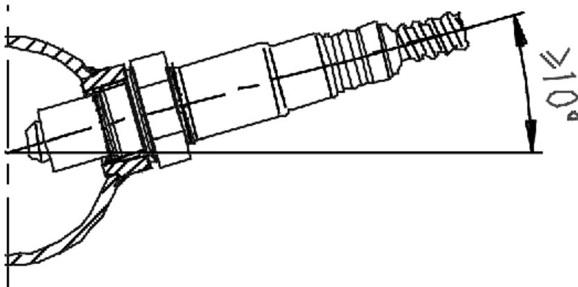
**Figure 8. Minimum mounting angle for the UEGO Sensor**
