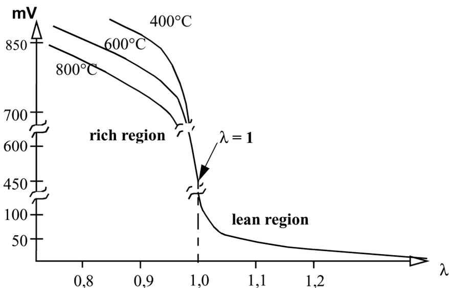
**Figure 1. Characteristic curve of a Nernst Cell O<sub>2</sub> Sensor**
