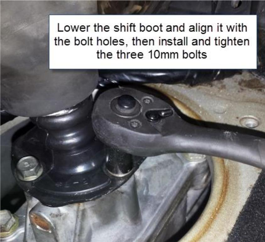
Lower the shift boot and align it with the bolt holes, then install and tighten the three 10mm bolts
