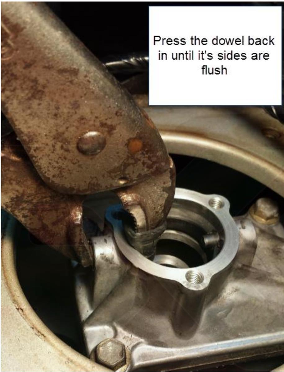
Press the dowel back in until it's sides are flush
