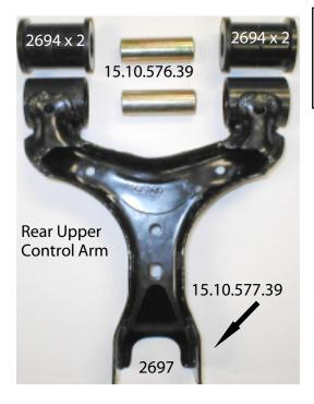
Remove the stock bushings from both control arms by pressing them out. Either hydraulic press or C-clamp with impact wrench. Thoroughly clean the inside of the control arm of any rubber residue Apply supplied Hyperlube to all urethane to metal contact points.
