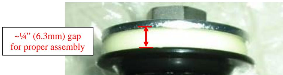
8. Ensure the gap is about 1/4" and the bushings are still centered in the shock mount. This verifies the bushings have been properly compressed.
