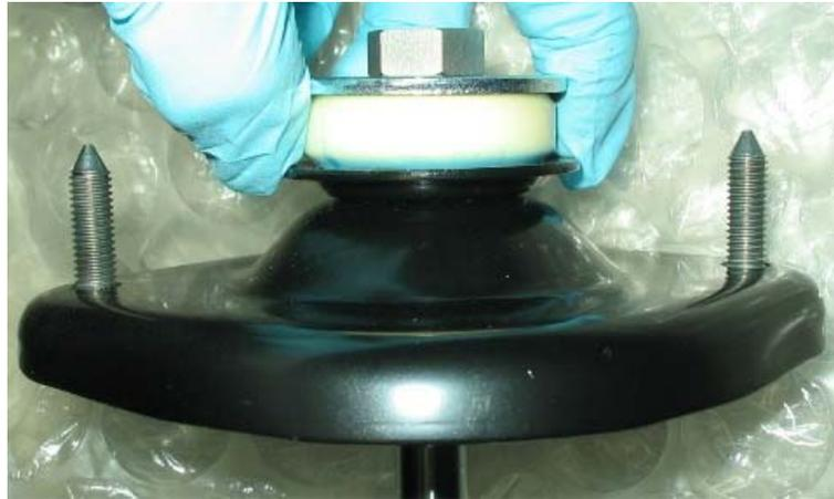
Tightening the M10 or M12 shoulder nut.
