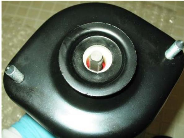
Installation of upper bushing, bushing centering during tightening
