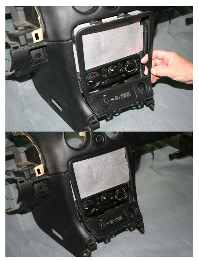
11. With the bezel installed, it should press fairly flush to the plate. If it is not flush, try trimming the tabs again to get a better fit. The bezel should snap in with minimal effort. If it feels like it's just not snapping in like it should, further trimming of the bezel tabs might be needed
