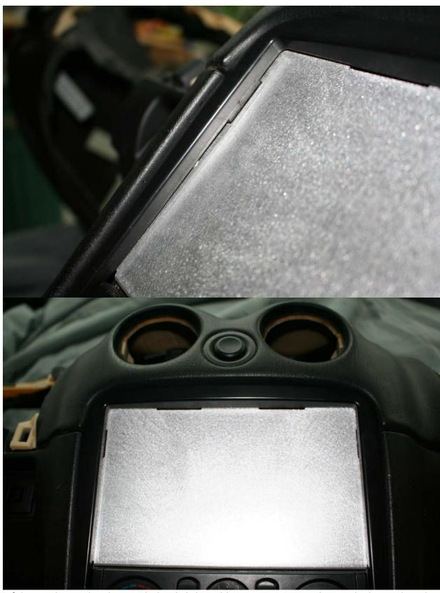
The edge of the notches in the plate might be slightly visible on some cars at a low angle due to the tolerance allowance built into the plates. You should not see them when sitting in the car with the way they are angle
