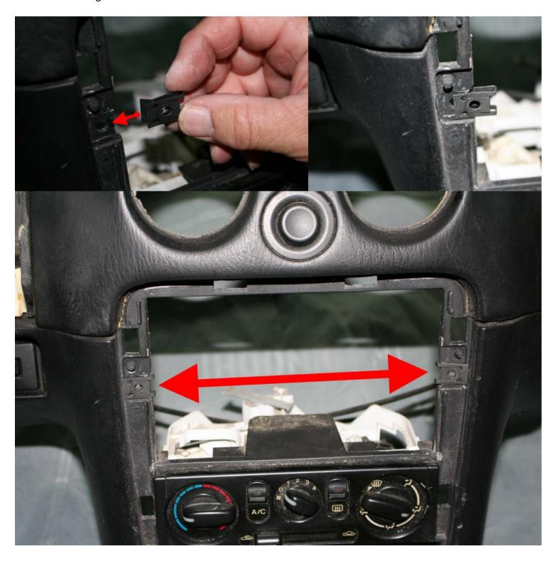
7. Find the two phillips head screws and plastic spacers. Push the screws through the two holes on the plate, and then slide the spacer over the back side of the screw. The spacers ensure proper depth of the plate. Snug the plate by screwing it into the threaded clips in the bezel recess, but do not tighten. If the top of the plate does not seat properly, you might need to trim more of the dash pad outline in step 5
