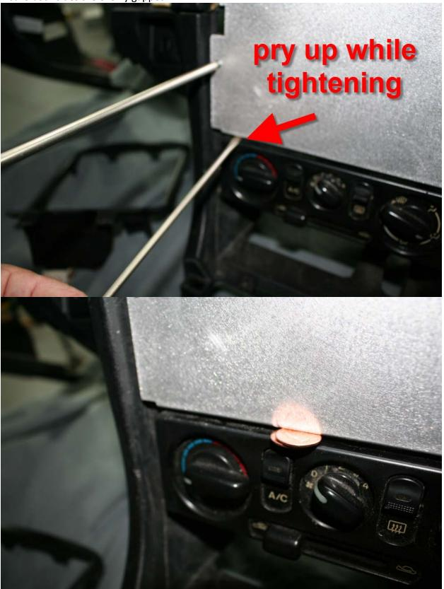
9. The plate should be installed firmly at this point.
