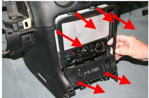
4. Once the bezel is removed, there might be a horizontal plastic bar spanning from side to side that must be removed. Some models might not have it (our 99 did, our 2002 did not). If it is present, remove it by twisting it off or snipping it with a pair of cutters
