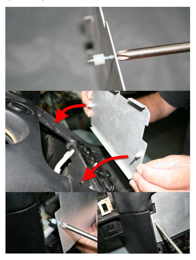
8. Take a flat head screwdriver and gently pry up on the gap on the bottom of the plate. This gap is important to set and can be checked correctly if the two pennies fit snugly. You'll want to make sure both sides are evenly gapped
