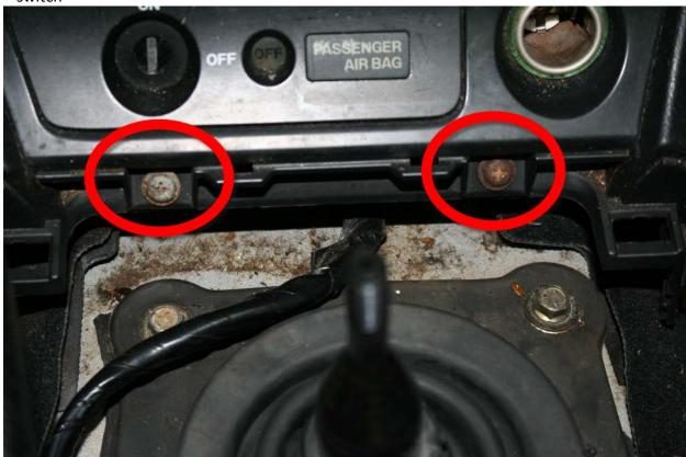
3. Remove radio bezel by grabbing it from the bottom, then pulling it evenly towards the shifter. Take care not to bend it or pull it from only one spot, but rather distribute the pull-load evenly across the stronger points of the bezel
