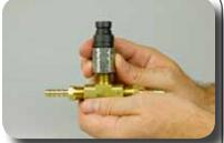
Attach flat face nipple (4) to the middle tee thread.
