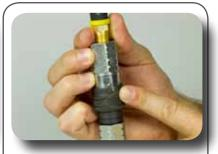
Turn the coupler's collar to lock it. After unlocked, retreact the coupler's head to disconnect the union
